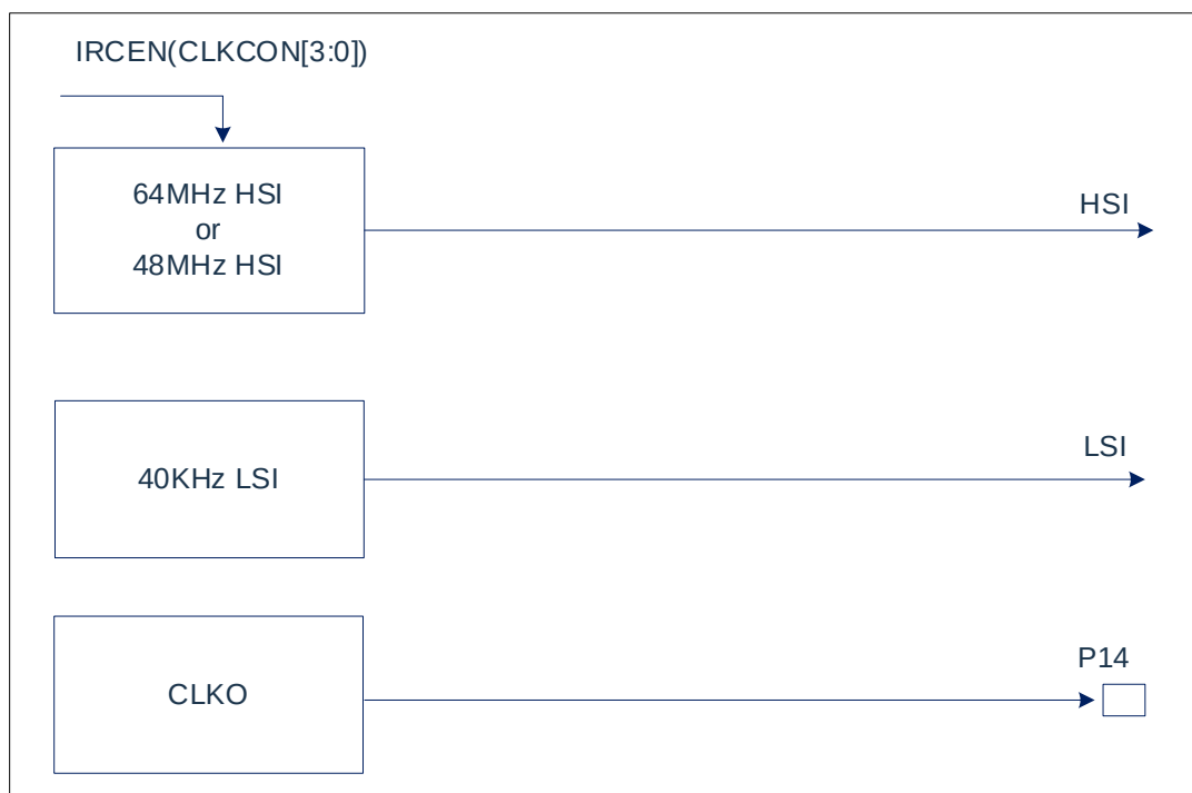
Figure3-1: Block diagram of the clock structure
